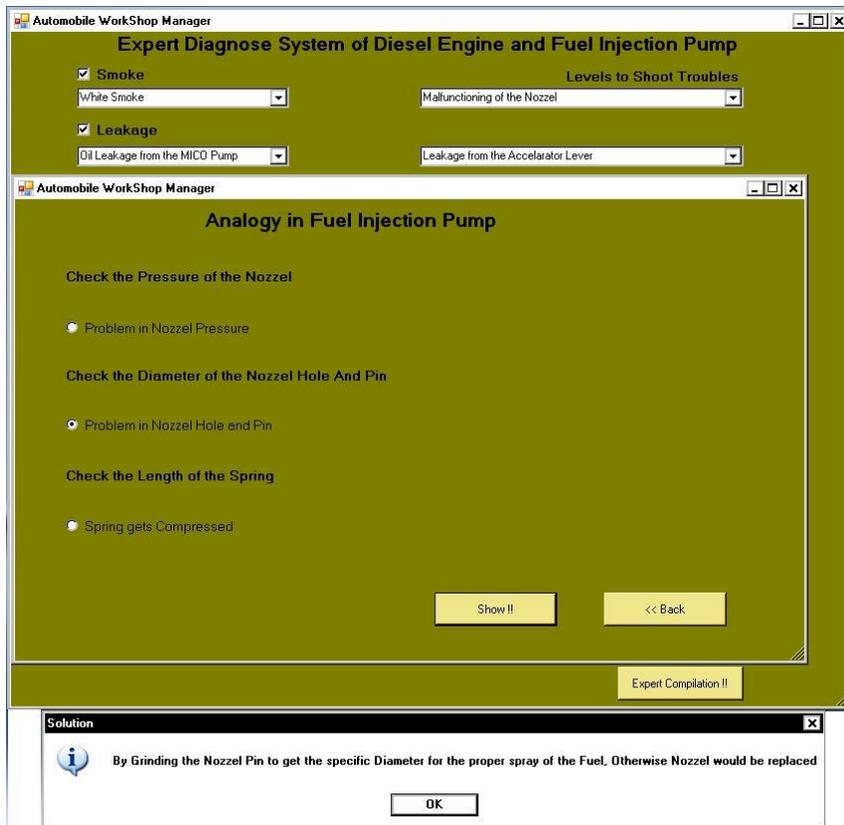
Fig. 4: Multiple selection & Solution Window
